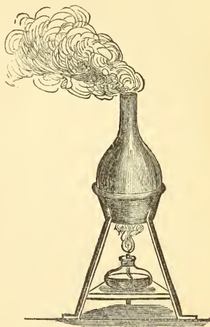
FIG. 31.—Apparatus for generating Chlorine Gas as a purifier of Buildings.
